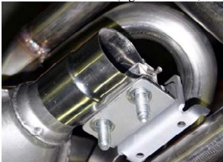
Slip the angled tailpipe section into the outlet end of the muffler's slipjoint sleeve clamp and tighten up the clamps' bolts enough to hold the joint from slipping apart. The angled end of the tailpipe as-built should slope slightly downward and to the rear.
