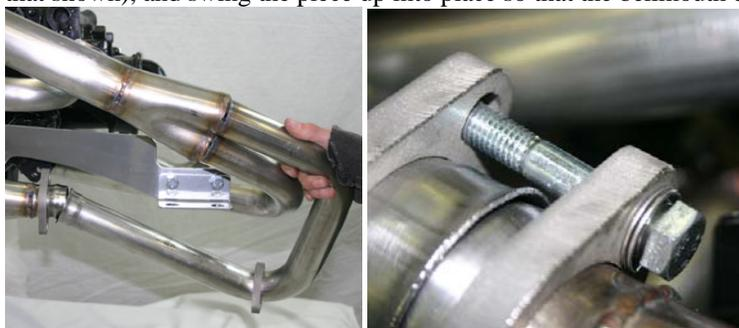
You will use the M8 x 45mm hexbolts with two of the conical Belleville washers stacked under each bolt head, and the flanged copper nuts with no washers to pull the captive flanges together, as shown above right.
