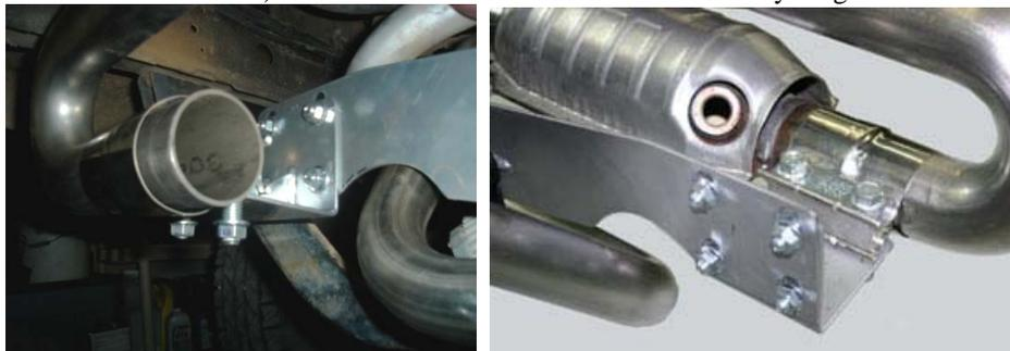
Another band clamp should be slipped in the opposite direction onto the 2" collector pipe end of the secondary. The clamp's bolts should be to the rear and the nuts downward so they will be easier to access. Next slide the J-pipe to the left enough that you can slip the longer leg of the J-pipe and the end of the secondary pair together.
