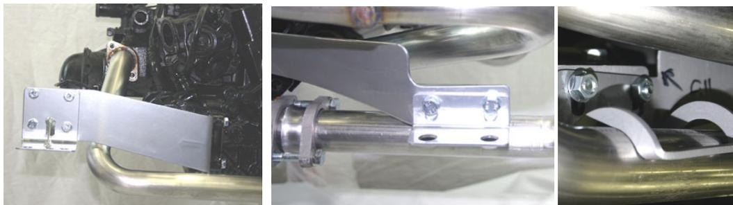
**5.** Do the same with the rightside main support bracket and attach the tailpipe shelf bracket and secondary pipe support saddle bracket to it as shown above center and above right (secondary pipe is in place in these pics).
