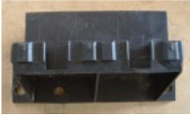
On '86 and later vans, the Idle Speed Control Unit (ISCU) is mounted to the front wall of the pillar cavity (it looks like a double-width relay box). Remove the controller still attached to its base connector by sliding the connector up and out of the plastic mounting bracket. Swing the controller out of the way, then remove the two screws that hold the plastic mounting bracket to the front wall of the cavity.
