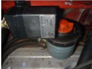
Then drill two holes and use the bracket's two screws to attach the base to the rear of the engine bay like in the picture far left. Swing the controller on the end of its wiring harness out across and pop it back into place in the mounting
