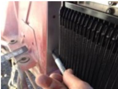
While holding the assembly in this position, mark where the two screw holes are in the forward cooler support plate. Use a marker or bent scribe to make center marks for the two holes that are against the cavity forward wall.
