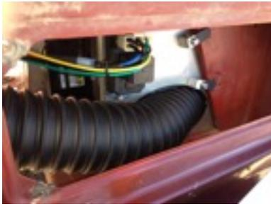
There is some variance in the sizing of the air filter inlet spigots, so if the duct hose won't "screw" on over the spigot, and you haven't used the 3" piece of 2" ABS pipe to connect to the snorkel tube, push the ABS pipe into the inlet spigot of the air filter housing, until it will stay in place by friction-fit. Then attach the duct hose to the ABS pipe and clamp in place.
