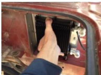
The cooler/fan assembly will be mounted within the D-pillar cavity, with both its hose fittings facing to the rear.
