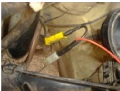
If the van doesn't have P/S or doesn't have a P/S pressure switch, you will connect the yellow wire inline with the fuel pump power connector. The fuel pump power wire exits the engine bay thru a small opening in the right-forward corner, directly forward of the air filter housing. Find the fuel pump power wire connector there, disconnect, and connect the male and female connectors of the yellow oil cooler power wire adapter inline., as is shown in the picture at left.
