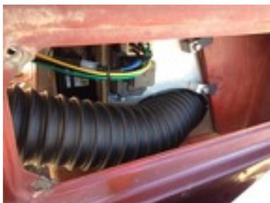
The black wire with small ring terminal is grounded; it can attach to any of the alternator chassis thru-bolts, there are several around the perimeter of the chassis. Slip the ring terminal over the bolt end and secure with the M5 nut and washer provided.
