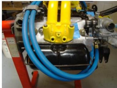
Now run the free ends of both hoses across the engine bay at an angle toward the support bracket as shown at far left, and lay both hoses in the bracket saddles. Lay the upper bracket saddle piece over both hoses, fit the top cover and bolt, and run the bolt down just enough to hold it all together. Then route the free ends of the hoses in a curve around the left end of the engine and thread them onto the banjo adapter fittings. It doesn't matter which hose goes where on the sandwich adapter.
