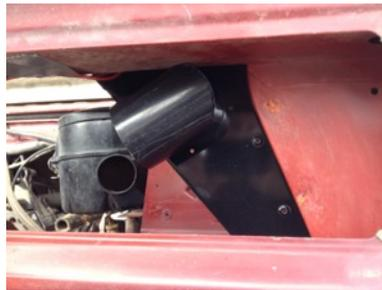
Position the rear support plate within the cavity box by leaning it forward as at far left, and tilting it upright so that the square notch in the top of the plate goes under the box beam on the roof of the cavity. In final position it should be vertical and backed up against the body gusset visible thru the taillight opening as shown at left.
