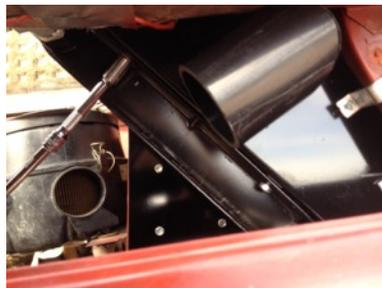
With the two #6x1/2" hexhead sheet metal screws, attach the rear support plate retaining tabs to the rivets in the plate, the screws will self-tap into the rivets. Position the tabs over the body gusset as shown in the picture far left, and tighten the screws just enough to hold the support plate loosely in place.
