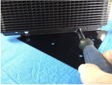
Attach the forward cooler support plate to the cooler with two of the #10x1/2" hexhead sheet-metal screws as in the photo far left. Snug the screws and then loosen them slightly to allow some movement to aid in positioning the cooler.
