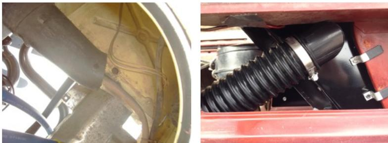
**Fit Intake Air Duct Hose:** The air filter housing's inlet horn has to be cut off partly to fit the intake air flex hose to it. Saw off the curved end of the inlet horn just after the start of the curve. The altered air horn will look like the picture at far left.
